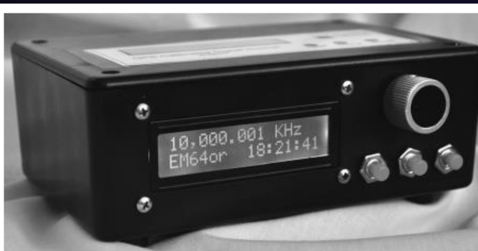
Figure 2 — Here is a completed VFO project, housed in a plastic project box. The Resolution, Band Select, and Reset pushbutton controls are located just below the rotary encoder.
